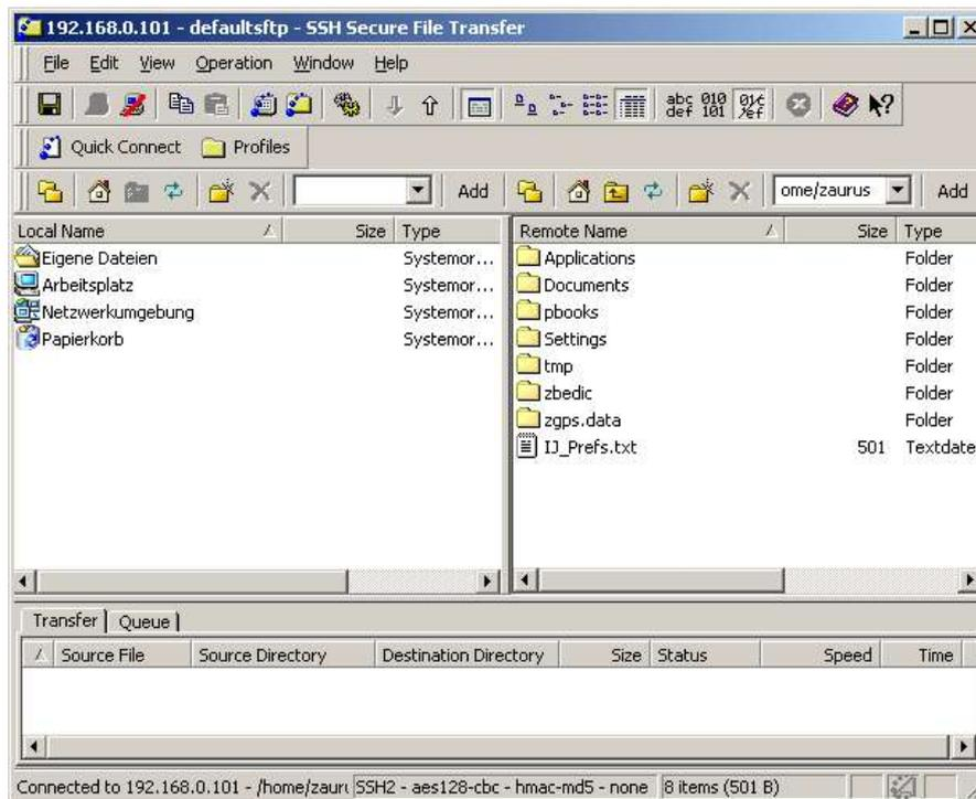
Figure 2: Screenshot of Secure File Transfer Client with connection from a Windows-client to a Zaurus-server
