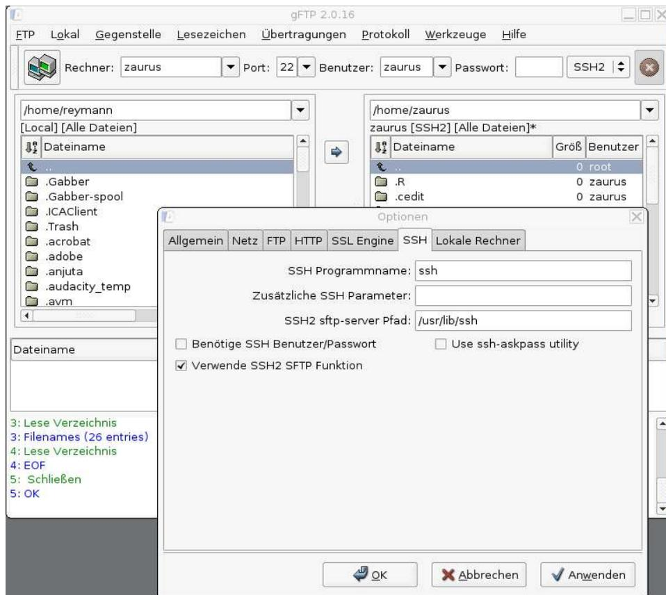
Figure 1: Screenshot of gftp with Options-Tab showing a connection from a GNU/Linux-desktop as client to a Zaurus as server
